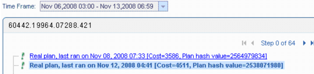
Figure 9: Two plans for the same query. The second plan has a 20% higher cost
